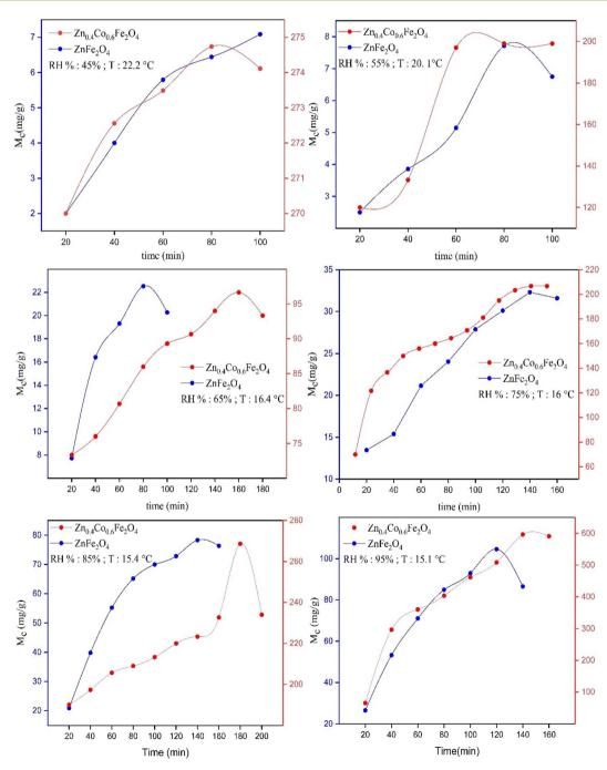
Graphs of moisture content ( $M_c$ ) versus time for synthesized ZnFe<sub>2</sub>O<sub>4</sub> and Zn<sub>0.4</sub>Co<sub>0.6</sub>Fe<sub>2</sub>O<sub>4</sub> at different RH percentages.
