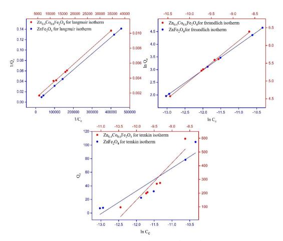
Fig. 6 Fitting of experimental data to various isotherm models for ZnFe<sub>2</sub>O<sub>4</sub> and Zn<sub>0.4</sub>Co<sub>0.6</sub>Fe<sub>2</sub>O<sub>4</sub>.
