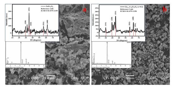
Fig. 2 Scanning electron micrographs along with X-ray diffraction patterns and energy dispersive X-ray spectra for (a)  $ZnFe_2O_4$  and (b)  $Zn_{0.4}Co_{0.6}Fe_2O_4$ .
