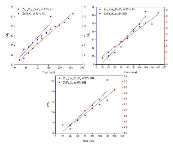
Fig. 7 Fitting of experimental data to a pseudo second-order kinetic model for  $ZnFe_2O_4$  and  $Zn_{0.4}Co_{0.6}Fe_2O_4$  at 75%, 85%, and 95% RH.
