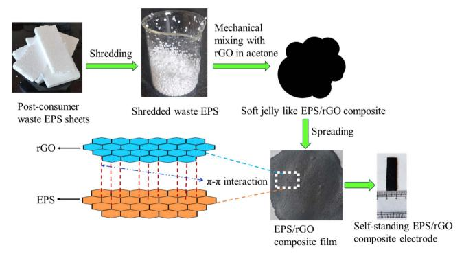
Fig. 1 Schematic representation of EPS/rGO electrode fabrication.
