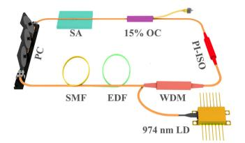
Fig. 5 Schematic diagram of the mode-looked erbium-doped fiber laser.
