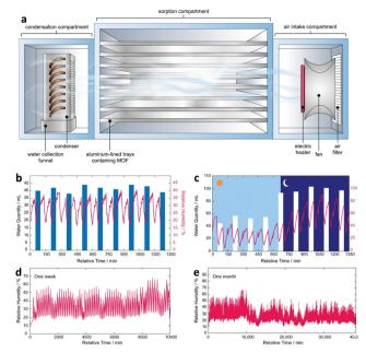
Fig. 13 (a) Schematic of the atmospheric water harvester. (b) Stress test for 24 h performed under a controlled environment (20% RH and 25 °C). (c) Assessment of real-world performance over a full day. (d) Realenvironment continuous performance for one week. (e) Performance of self-adaptive water harvesting devices during continuous operation for a month. Reproduced with permission from ref. 109. Copyright 2022, The Author(s).
