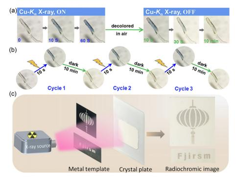
Fig. 3 Radiochromic behavior for RCS-2: (a) time-dependent images for crystalline samples of RCS-2 upon irradiation of Cu-K<sub>rr</sub> X-rays. (b) Colored-decolored cycles of a single-crystal sample upon irradiation of Cu-K<sub>u</sub>. (c) Radiochromism imaging. (The photographs of (a) and (b) were both captured in their original context.)
