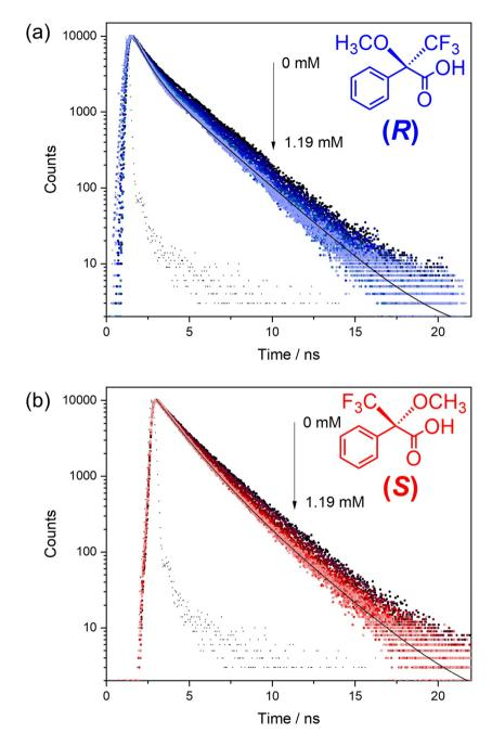
Fig. 4 Fluorescence decay curves for the BINOL fluorophore in acetonitrile alone (10 mM) and in the presence of an increasing concentration of (a) (R)-Mosher's Acid or (b) (S)-Mosher's Acid. The fluorescence was recorded using  $l_{ex}$  = 300 nm and  $\lambda_{em}$  = 416 nm. The solid black line is the fit and the black data points the instrument response function (IRF).
