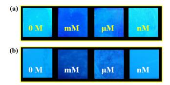
Fig. 7 Detection of various concentrations of (a)  ${\rm Hg^{2+}}$  and (b) ranitidine using the MOF@PVDF-PVP thin film composite.
