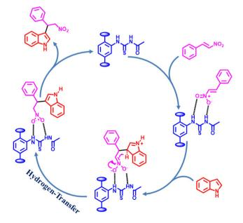
Scheme 2 Proposed mechanism for the Friedel-Crafts alkylation between IND and NS using 1' as a catalyst.
