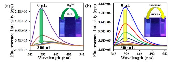
Fig. 2 Change in the fluorescence intensity of 1' after incremental addition of (a) 10 mM Hg<sup>2+</sup> and (b) 5 mM ranitidine solutions in aqueous and HEPES buffer media, respectively.
