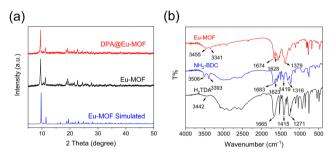
Fig. 2 (a) PXRD patterns of Eu-MOF, simulated Eu-MOF, and DPA@Eu-MOF. (b) FT-IR spectra of Eu-MOF, NH<sub>2</sub>-BDC and H<sub>2</sub>TDA.
