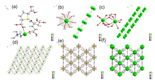
Fig. 1 Crystal structures of Eu-MOF. (a) Asymmetrical unit of Eu-MOF. (b) Coordination environment of Eu<sup>3+</sup> and 1D structure in the b-axis of Eu-MOF. (c) The [Eu<sub>2</sub>(COO)<sub>3</sub>] dinuclear cluster structural unit and 1D in the c-axis of Eu-MOF. (d) 2D structure of Eu-MOF from ac plane. (e) 2D structure of Eu-MOF from ab plane. (f) 3D framework of Eu-MOF.
