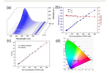
Fig. 3 (a) Fluorescence spectra of Eu-MOF with 0 to 500  $\mu$ M DPA. (b) Relationship between luminescence intensity of 434 and 619 nm versus DPA concentration. (c) Standard curve of  $\Delta(I_{434}/I_{621})$  versus DPA concentration. (d) CIE chromaticity diagram of Eu-MOF in the presence of 0 to 500 μM DPA.
