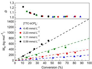
Fig. 3 Evolution of  $M_n$  and D during PI-RAFT bulk polymerisation of nBA for different targeted molar masses. Dashed lines represent the theoreotical molar masses.
