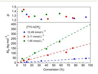
Fig. 2 Evolution of  $M_n$  and  $\mathcal{D}$  during PI-RAFT polymerisation of MMA for different targeted molar masses. Dashed lines represent the theoretical molar masses.
