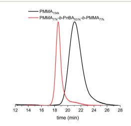
Fig. 4 SEC-RI chromatograms of PMMA<sub>154k</sub> and the corresponding PMMA<sub>77k</sub>-b-PnBA<sub>531k</sub>-b-PMMA<sub>77k</sub> triblock copolymer.
