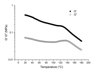
Fig. 5 Temperature dependence of G' and G'' of PMMA<sub>77k</sub>-b-PnBA<sub>531k</sub>-b-PMMA<sub>77k</sub> triblock copolymer from 20 to 180 °C.
