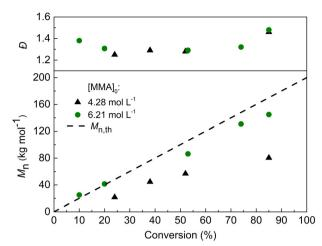
Fig. 1 Evolution of  $M_n$  and  $\mathcal{D}$  during PI-RAFT polymerisation at ambient temperature with different concentrations of MMA in acetonitrile.
