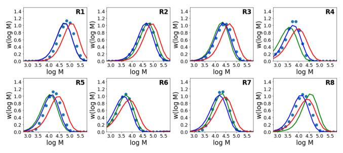
Fig. 5 Molecular weight distribution of the final sample for experimental data (circles), in comparison to the distributions predicted by the kinetic model (red), a purely data-driven neural network (green), and a PCINN (blue).
