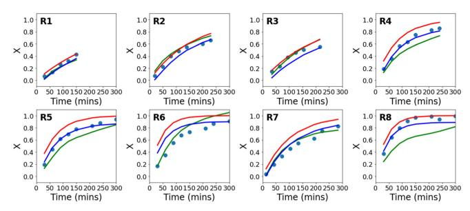
Fig. 3 Evolution of conversion with time for experimental data (circles), in comparison to the theoretical evolution of conversion following eqn (16) (red), a conventional neural network (green), and a PCINN (blue).
