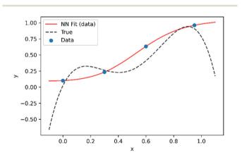
**Fig. 1** Example of a neural network model (red line) fit to a series of four (x,y) data points extracted from an underlying distribution given by  $y = -18x^4 + 35x^3 - 21x^2 + 4.4x$  (dotted black line).
