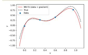
Fig. 2 Demonstration of approach to combine data and theory in training neural network. As opposed to Fig. 1, in addition to the data points it is assumed that the data follows a trend represented by  $y = -23x^4 + 47x^3 - 20x^2 + 6.6x$  which is used to supply the values of dy/dx<sub>theo</sub> in eqn (2).
