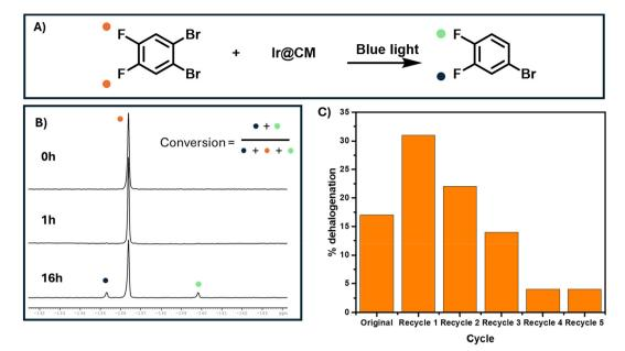
Fig. 7 (A) Reaction scheme of dehalogenation; (B) <sup>19</sup>F NMR of reaction mixture at different time points. Debromination is indicated by the appearance of two peaks at –135.25 ppm and –139.75 ppm. (C) Dehalogenation efficiency of pbtz-Ir@CM over numerous cycles determined by integration of peaks at –135.25 ppm and –139.75 ppm against 1,2-dibromo-4,5-difluorobenzene peak at –136.4 ppm.
