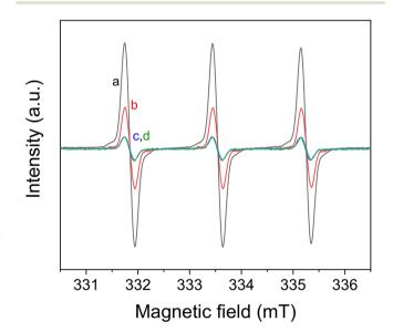
**Fig. 2** Electron paramagnetic resonance (EPR) spin trapping spectra of TEMP  $^1O_2$  generated under different conditions. (a) Eosin Y disodium salt (1 mg mL $^{-1}$ ), tetramethylpiperidine (TEMP, 0.1 M),  $O_2$ . (b) Eosin Y disodium salt (1 mg mL $^{-1}$ ), TEMP (0.1 M), air. (c) TEMP (0.1 M),  $O_2$ . (d) Eosin Y disodium salt (1 mg mL $^{-1}$ ), TEMP (0.1 M),  $O_2$ , darkness. All the samples were irradiated with a blue LED for 30 min before measurement.
