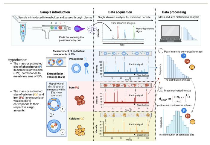
Fig. 5 Hypothetical composition of DEVs showing phosphorus (P) distribution on the membrane area and calcium (Ca) and iron (Fe) distribution within the cargo, with two hypothetical distribution scenarios. Size measurements of elements were conducted using single-element analysis with SP-ICP-MS and mass-to-size conventions.
