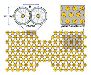
Fig. 1 The PGPNs are composed of gold nanoparticle cores with radius  $r_0 = 25$  nm and f = 900 polymers grafted on their surface. The pair interactions between the PGPNs help them to form a stable cross-linked network. Equilibrated double notched PGPNs arranged in a hexagonal lattice are stable and form gold nanoclusters with dipole moments that depend on the interaction between the PGPNs that form the array.
