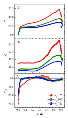
Fig. 4 Average forces per unit thickness,  $\sigma = F/W$ , on the right edge of the PGPN arrays along the direction of stretching as a function of strain at constant pulling velocity,  $u = 0.001u_0$ , and  $E = 39k_BT$ . (a) The net force,  $\sigma_x$ :  $F_x/W$ , (b) bonded contributions,  $\sigma_b^x$ :  $F_b/W$  and (c) non-bonded contributions,  $\sigma_b^x$ :  $(F_{nb}^{rep} + F_{nb}^{rob})/W$ .
