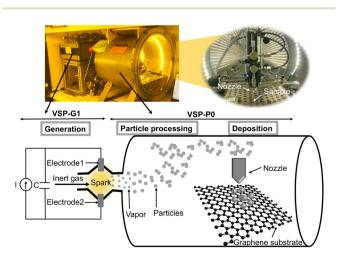
Fig. 2 Schematic view of the spark ablation method system (VSPARTICLE BV, the Netherlands) used for NP printing.
