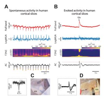
**Fig. 6** Graphene microtransistors for measuring human cortical activity. Spontaneous (A; left) and evoked (B; right) activity from human cortical slices *in vitro* recorded with graphene microtransistors. Traces of full-band signals (red), firing rate or logMUA in arbritary units (blue), spectogram and AC component of the signal (black). In the inset, single detected events are overlapped. C and D represent the experimental set-up with the overlapping anatomical reconstructions.
