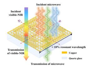
Fig. 1 Schematic of the MMFSM.
