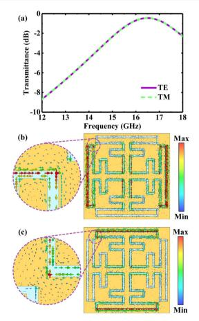
Fig. 3 (a) Simulated transmittance of the MFSM in the Ku band (12-18 GHz) at normal incidence under TE and TM polarization. (b and c) Simulated surface current density of the MFSM at its resonant frequency (16.5 GHz) under (a) TE polarization and (b) TM polarization. Insets in (b) and (c) are the amplified surface current density of the corresponding purple dotted circle regions.
