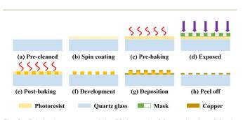
Fig. 8 Fabrication process of the FSM sample: (a) pre-cleaning; (b) spin coating; (c) pre-baking; (d) exposure; (e) post-baking; (f) development; (g) deposition; (h) peeling off.
