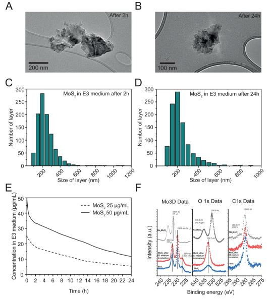
Fig. 1 Characterization of exfoliated MoS<sub>2</sub>. (A) HRTEM images after 2 hours and (B) 24 hours and corresponding layer size distributions in E3 medium after 2 hours (C) and 24 hours (D). (E) Colloidal stability of  $MoS_2$  in zebrafish E3 medium at 25 and 50  $\mu$ g mL<sup>-1</sup> during 24 h. (F) Signals from XPS analyses before (blue traces) and after 24 hours exposure to E3 medium (red traces). Molybdate salt (black traces) was used as reference control.
