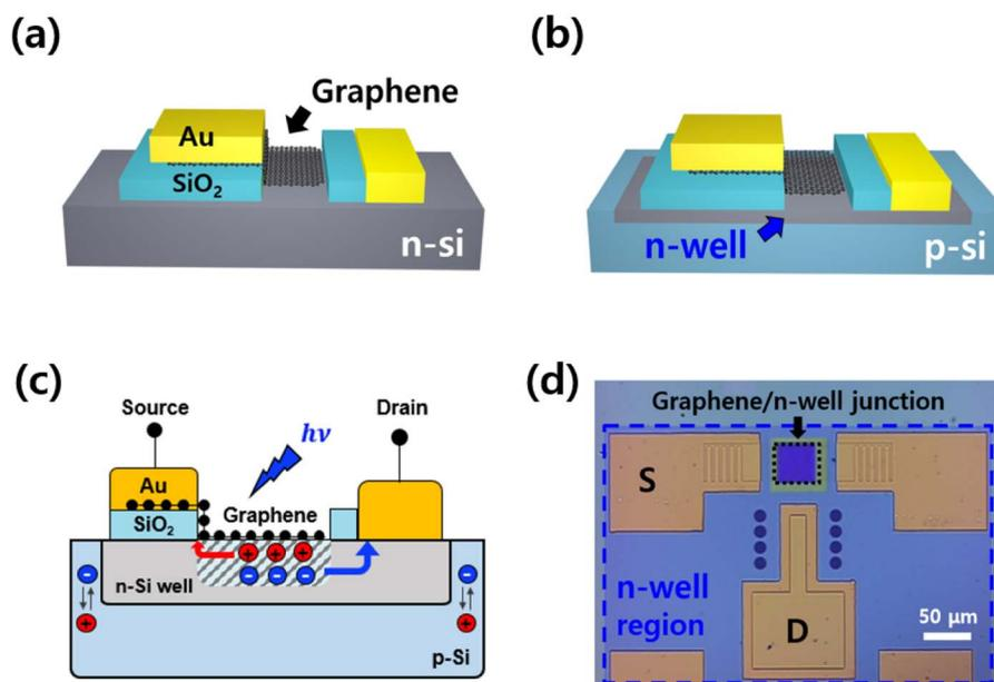
Fig. 1 Schematic diagrams of (a) graphene/n-type bulk Si Schottky junction photodetector and (b) graphene/n-Si well-tub/p-Si photodetector. (c) A cross-sectional schematic of the device including the isolated well-tub structure. After the implantation process, the annealing time was varied to split the n-Si well depth. (d) Optical image of fabricated the device (black dashed rectangle: graphene/n-Si well junction area, blue dashed rectangle: n-Si well region).
