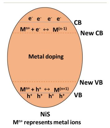
Fig. 8 Schematic illustration of band structure modification due to metal doping.
