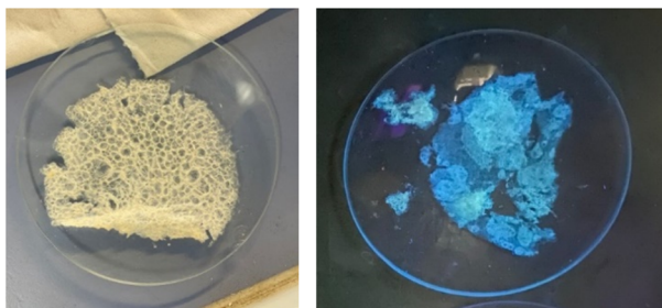
Fig. 2 (Left) Film 1-PTH obtained. (Right) Film 1-PTH under UV light (364 nm).
