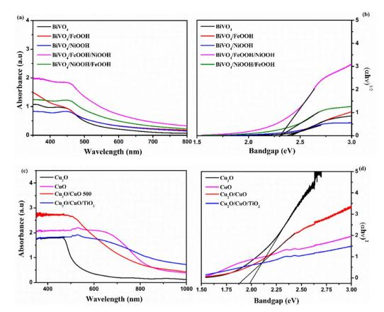
Fig. 4 (a and c) UV-vis absorption spectra. (b and d) Tauc's plot of  $BiVO_4$ ,  $BiVO_4$ /FeOOH,  $BiVO_4$ /NiOOH,  $BiVO_4$ /FeOOH/NiOOH and  $BiVO_4$ /NiOOH/FeOOH nanostructured photoanodes and  $Cu_2O$ ,  $Cu_2O$ /CuO, (inset)  $Cu_2O$ /CuO/TiO<sub>2</sub> and CuO photocathodes.
