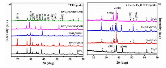
Fig. 2 XRD pattern of (a)  $BiVO_4$ ,  $BiVO_4$ /FeOOH,  $BiVO_4$ /NiOOH,  $BiVO_4$ /FeOOH/NiOOH and  $BiVO_4$ /NiOOH/FeOOH nanostructured photo-anodes and (b)  $Cu_2O$ ,  $Cu_2O$ /CuO,  $Cu_2O$ /CuO/ $TiO_2$  and CuO photocathodes.
