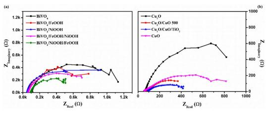
Fig. 6 Electrochemical impedance spectra (EIS) of (a)  $BiVO_4$ ,  $BiVO_4$ /FeOOH,  $BiVO_4$ /NiOOH,  $BiVO_4$ /FeOOH/NiOOH and  $BiVO_4$ /NiOOH/FeOOH photoanodes and (b)  $Cu_2O$ ,  $Cu_2O$ /CuO,  $Cu_2O$ /CuO/TiO<sub>2</sub> and CuO photocathodes tested in 0.1 M  $Na_2SO_4$  (pH 6) in AM 1.5 G equipped illumination source with a power intensity of 100 mW cm<sup>-2</sup>.
