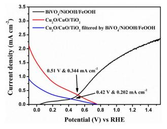
Fig. 8 Overlay of the absolute LSV responses of BiVO<sub>4</sub>, BiVO<sub>4</sub>/ NiOOH/FeOOH, Cu<sub>2</sub>O and Cu<sub>2</sub>O/CuO/TiO<sub>2</sub> to find the operating point of the tandem cell.
