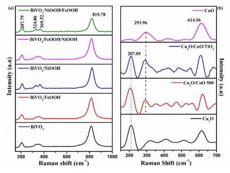
Fig. 3 (a) Raman vibrational spectra of (a) BiVO<sub>4</sub>/, BiVO<sub>4</sub>/FeOOH, BiVO<sub>4</sub>/NiOOH, BiVO<sub>4</sub>/FeOOH/NiOOH and BiVO<sub>4</sub>/NiOOH/FeOOH nanostructured photoanodes and (b) Cu<sub>2</sub>O, Cu<sub>2</sub>O/CuO, Cu<sub>2</sub>O/CuO/TiO<sub>2</sub> and CuO photocathodes.
