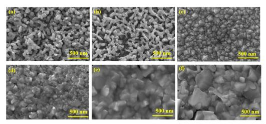
Fig. 1 FESEM image of (a)  $BiVO_4$ , (b)  $BiVO_4$ /NiOOH/FeOOH nanostructured photoanodes, (c) pure  $Cu_2O$ , (d)  $Cu_2O$ /CuO, (e)  $Cu_2O$ /CuO/ $TiO_2$  and (f) CuO photocathode.
