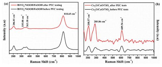
Fig. 11 Raman spectra obtained before and after PEC testing of (a) the BiVO<sub>4</sub>/NiOOH/FeOOH photoanode and (b) Cu<sub>2</sub>O/CuO/TiO<sub>2</sub> photocathode
