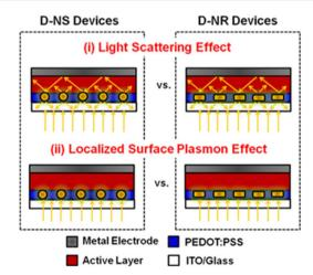
Fig. 7 Schematic of two strategies for enhancing light trapping in PEDOT:PSS buffer layers: (i) FLS and (ii) LSPR effects. Reproduced from ref. 59 with permission from the American Chemical Society.
