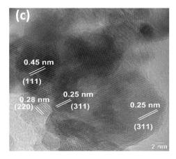
Fig. 3 (a) TEM of the CoFe<sub>2</sub>O<sub>4</sub> nanoparticles, (b) particle size distribution for CoFe<sub>2</sub>O<sub>4</sub> nanoparticles, and (c) HRTEM of the CoFe<sub>2</sub>O<sub>4</sub> nanoparticles.
