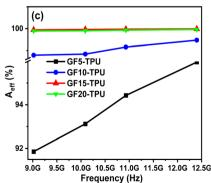
Fig. 7 (a) The comparison plot of the contribution of  $SE_{A}$ ,  $SE_{R}$  and  $SE_{T}$  for the developed GF–TPU nanocomposites, (b) power coefficients for the GF15–TPU nanocomposite, and (c)  $A_{eff}$  of the developed GF–TPU nanocomposites as a function of frequency.
