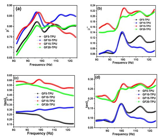
Fig. 10 (a) The real part of the permeability  $\mu'$ , (b) the imaginary part of permeability  $\mu''$ , (c) dielectric loss,  $\tan \delta_{\varepsilon}$ , and (d) magnetic loss,  $\tan \delta_{\mu}$ , as a function of the frequency for all the developed GF–TPU nanocomposites.
