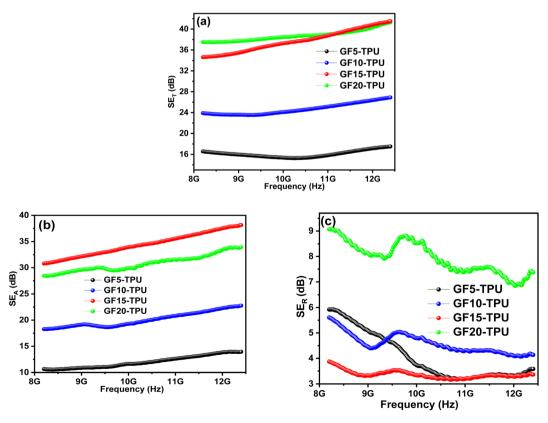
Fig. 6 EMI (a) total shielding effectiveness,  $SE_T$ , (b) shielding due to absorption,  $SE_A$ , and (c) shielding due to reflection  $SE_R$  as a function of frequency in the X-band range for the developed nanocomposites.
