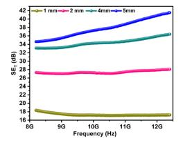
Fig. 8 The variation of SE<sub>T</sub> with tuned thickness as a function of frequency for the developed GF15-TPU nanocomposites.
