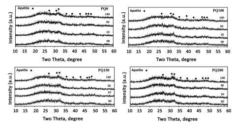
Fig. 7 XRD patterns of the different pastes before and after immersion in SBF solution for 1, 3, and 14 days.
