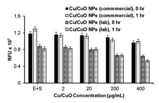
Fig. 3 A comparative hACE-2 enzyme inhibition study of laboratorysynthesized and commercially available Cu/CuO nanocomposites. The study was designed to understand the effect of concentrations and reaction periods.
