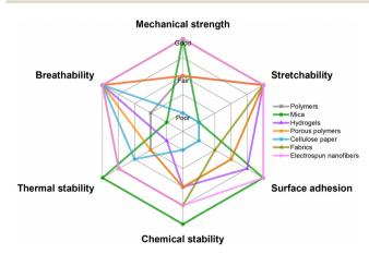
Fig. 2 Properties of different types of flexible substrates.
