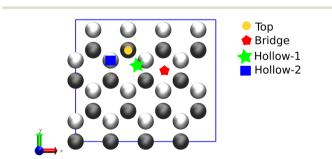
Fig. 7 Different adsorption sites at the Zn-{0001} plane. Top (yellow circle), bridge (red pentagon), hollow-1 (green star), and hollow-2 (blue square) represent the different possible adsorption sites. Gray-colored spheres: Zn surface; degraded color spheres: Zn under surface.
