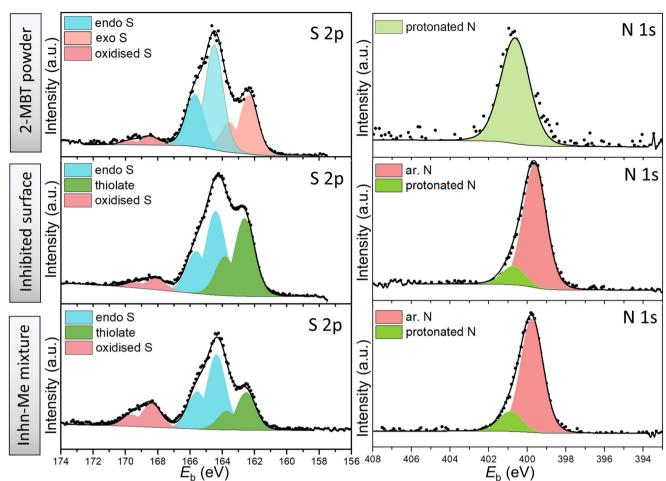
Fig. 6 High-resolution XPS spectra of S 2p and N 1s of 2-MBT powder (reference), ZE surface treated with 2-MBT and precipitates of inhibitor solution mixed with ZnCl<sub>2</sub>.
