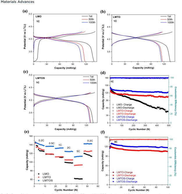
Fig. 8 Charge/discharge capacity profile of (a) LMO, (b) LMTO, and (c) LMTOS cathodes and (d) charge/discharge cycling performance of the three samples at cut-off voltages of 4.3–3.1 V (1C). (e) Rate performance of three cathodes from 4.3 to 3.1 V at different current densities, and (f) charge/discharge cycling performance of three cathodes at cut-off voltages of 4.3–3.1 V (5C).
