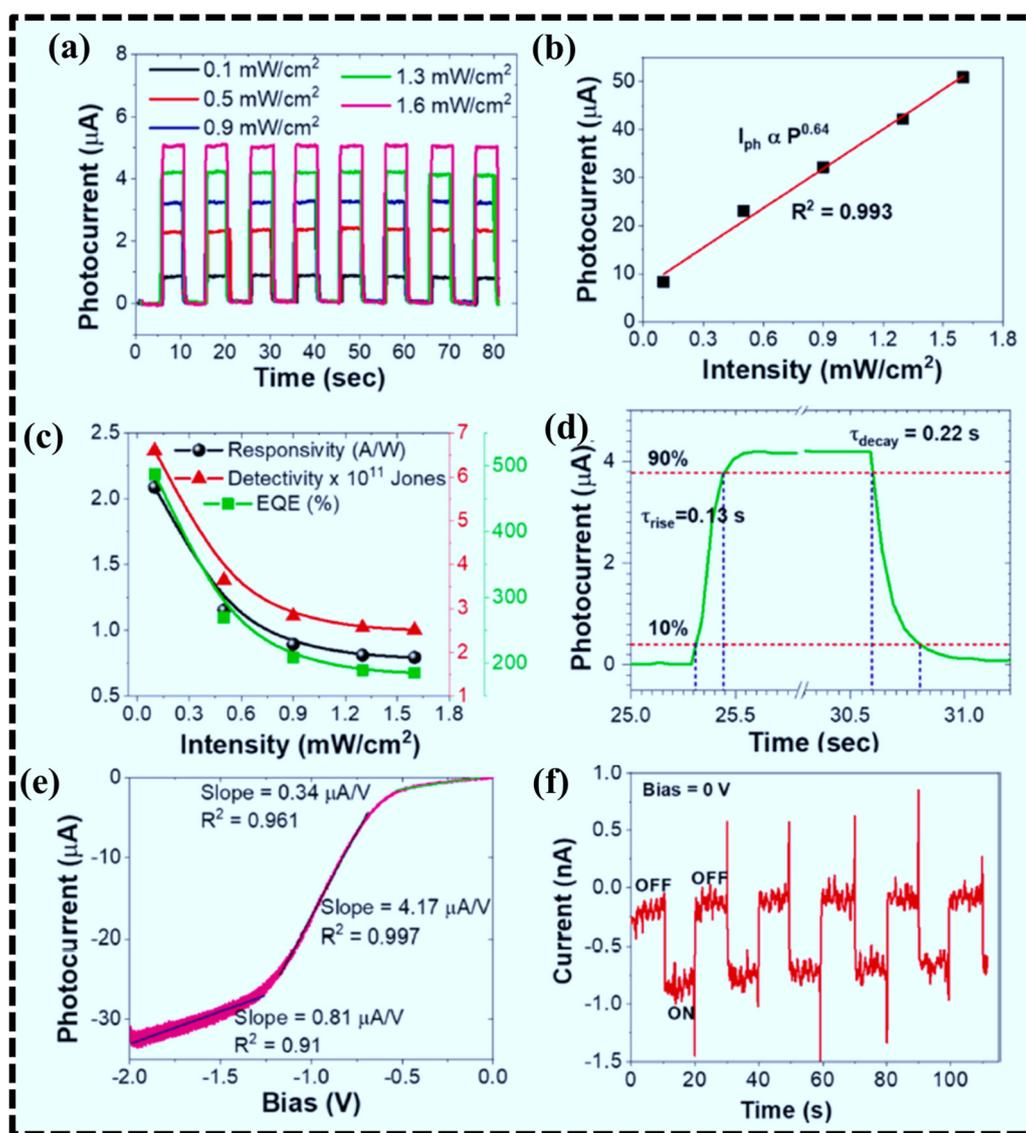
Fig. 11 (a) Time dependent photo response of the Ag-WS<sub>2</sub> photodetector device at different illumination intensities, (b) photocurrent with respect to the illumination intensities, (c) responsivity, detectivity and EQE of the photodetector device, (d) rise and decay time constant, (e) photocurrent with respect to the applied bias potential and (f) time dependent photo response under an applied bias potential of 0 V. Reprinted with permission from ref. 141, Copyright of Elsevier 2021.
