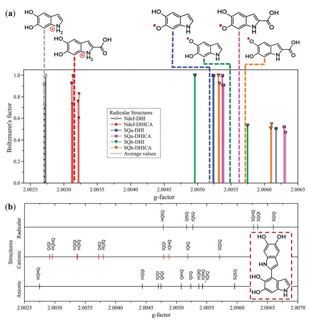
Fig. 8 Distribution of the theoretical g-values from eumelanin moieties that are: (a) radical monomers and (b) homo- and hetero-dimers. Compatible behavior was obtained for anionic and cationic monomers. The inset in (b) represents an example of a homo-dimer. Reproduced from A. Batagin-Neto et al. (2015)<sup>77</sup> with permission from the PCCP Owner Societies
