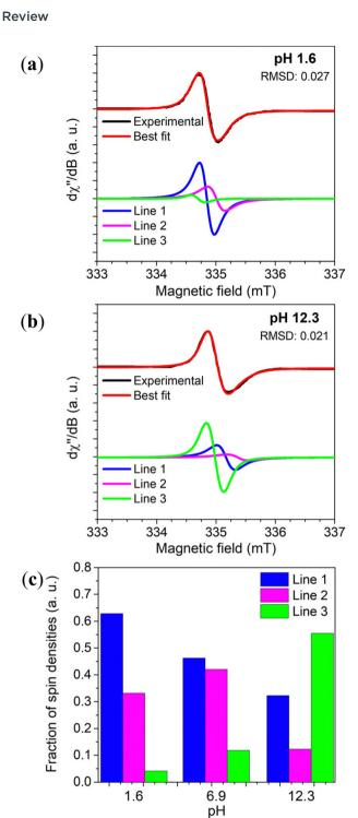
Fig. 6 Variation of Dopa-Eumelanin spin populations with pH obtained from X-band EPR spectrum simulation considering three different Voight lines. In (a) pH 1.6, and (b) pH 12.3. (c) The spin concentration estimation of the three-component fitting. Reproduced with permission from J.V. Paulin et al. (2019). Copyright © 2019, American Chemical Society.
