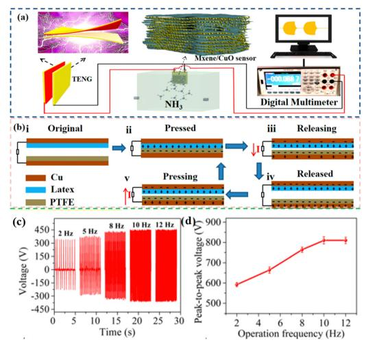
Fig. 5 (a) Schematic illustration of a self-powered  $NH_3$  sensor driven by a TENG. (b) The working mechanism of the TENG. (c) The open-circuit voltage of the TENG at different operating frequencies. (d) Variation trend of output voltage at different operating frequencies. The voltage/current variation. Reproduced from ref. 44 with permission from ACS Publications, copyright 2021.
