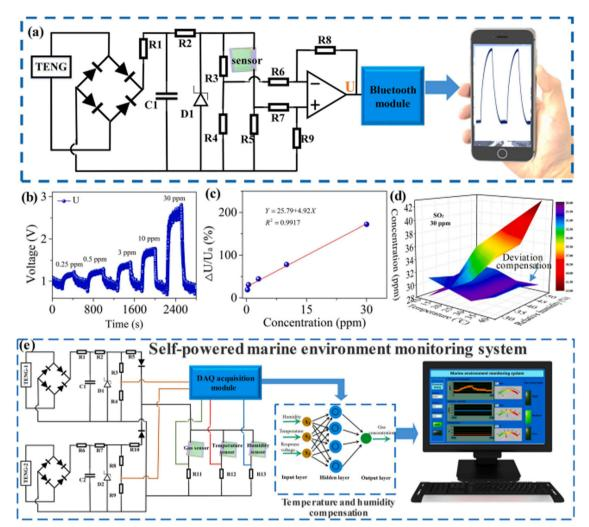
Fig. 3 (a) The wireless sensor detection circuit driven by the liquid-solid TENG. (b) The voltage values of U and (c) the voltage response ( $\Delta U/Ua$ ) at different SO<sub>2</sub> concentrations. (d) Comparison of sensor errors caused by temperature and humidity before and after correction. (e) The self-powered marine environment monitoring system. Reproduced from ref. 48 with permission from Elsevier, copyright 2022.
