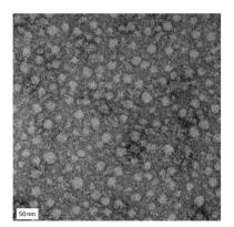
Fig. 5 TEM micrographs of GMA-EGDMA-S<sup>+</sup> give a mean particle diameter of 29  $\pm$  10 nm. The scale bar represents 50 nm.
