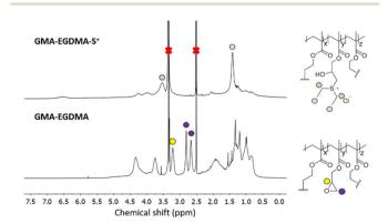
Fig. 3 <sup>1</sup>H NMR spectrum in DMSO-D6 (residual solvent signals are labelled with red crosses) of GMA-EGDMA-S<sup>+</sup>, with characteristic signals of the sulfonium group at  $\delta$  = 1.4 ppm labelled blue and at  $\delta$  = 3.5 ppm labelled green.
