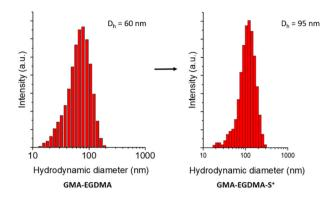
Fig. 4 The hydrodynamic diameters of GMA-EGDMA-S<sup>+</sup> (in 5 mM KCl) and GMA-EGDMA (in DCM) were measured by means of DLS indicating a semi bimodal size distribution. This increase in size is likely the result of same charges repelling each other as well as a difference in solvents.
