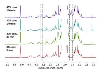
**Fig. 6** Conversion of epoxides during a ring-opening reaction of **GMA-EGDMA-S**<sup>+</sup> with 5 equiv. of diethyl sulfide in AcOH/acetone 1:1, as analyzed by <sup>1</sup>H NMR spectroscopy in acetone-d6. Conversion was calculated utilizing 1,3,5-trioxane as an internal standard. Its singlet peak can be seen at 5.1 ppm.
