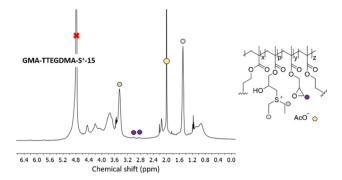
Fig. 8 <sup>1</sup>H NMR spectrum of GMA-TTEGDMA-S<sup>+</sup>-15 in D<sub>2</sub>O displays the characteristic sulfonium peaks at  $\delta$  = 1.4 ppm and  $\delta$  = 3.5 ppm along with the remaining epoxide peaks at  $\delta$  = 2.6 ppm and  $\delta$  = 2.8 ppm (the epoxide peak at  $\delta$  = 3.2 ppm is hidden under the methylene peaks of the sulfonium group). The acetate counter ion can also be seen at  $\delta$  = 1.9 ppm. The structure of the nanogel was simplified to enhance clarity.
