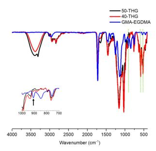
Fig. 9 IR spectrum of 50-THG and 40-THG. The green dotted lines over peaks at  $\nu = 585 \text{ cm}^{-1}$  and  $\nu = 632 \text{ cm}^{-1}$  highlight the emergence of S<sup>+</sup>-C vibrational stretches. The green dotted line (and arrow in the inset) at  $\nu = 907 \text{ cm}^{-1}$  specifies the disappearance of epoxide moieties demonstrating a successful reaction.
