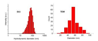
Fig. 2 GMA-EGDMA nanogel at 31% monomer conversion was analyzed by DLS and TEM displaying unimodal distribution for both
