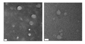
Fig. 10 TEM images of 50-THG (left) and 40-THG (right) indicate the formation of spherical particles with high polydispersity. The scale bars represent 50 nm. 40-THG had a particle diameter of 79 + 56 nm and 50-THG had a particle diameter of 61 ± 17 nm.
