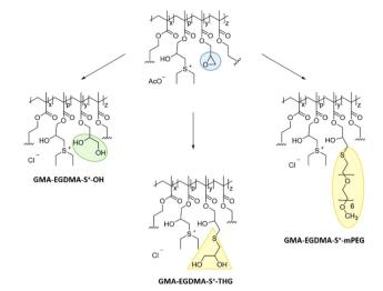
Scheme 2 A schematic overview of the attempts made to achieve water-soluble GMA-EGDMA-S<sup>+</sup>-x. Hydrolysis of the remaining epoxides with TFA to form GMA-EGDMA-S<sup>+</sup>-OH was attempted as well as ring opening reactions with hydrophilic thiols to GMA-EGDMA-S<sup>+</sup>-THG and GMA-EGDMA-S<sup>+</sup>-mPEG.
