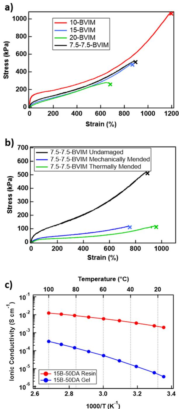
**Fig. 2** Characterization of ionic liquid gels. (a) Tensile strength of gels with varying amounts of copolymer. (b) Tensile experiments of formulation 7.5-7.5-BVIM after printing, after being cut and mechanically mended (pushed together), and after being thermally mended at 85 °C. (c) Electrical Impedance Spectroscopy (EIS) data of formulation 7.5-7.5-BVIM as a resin (red) and after printing (blue) over a range of temperatures (20-100 °C).
