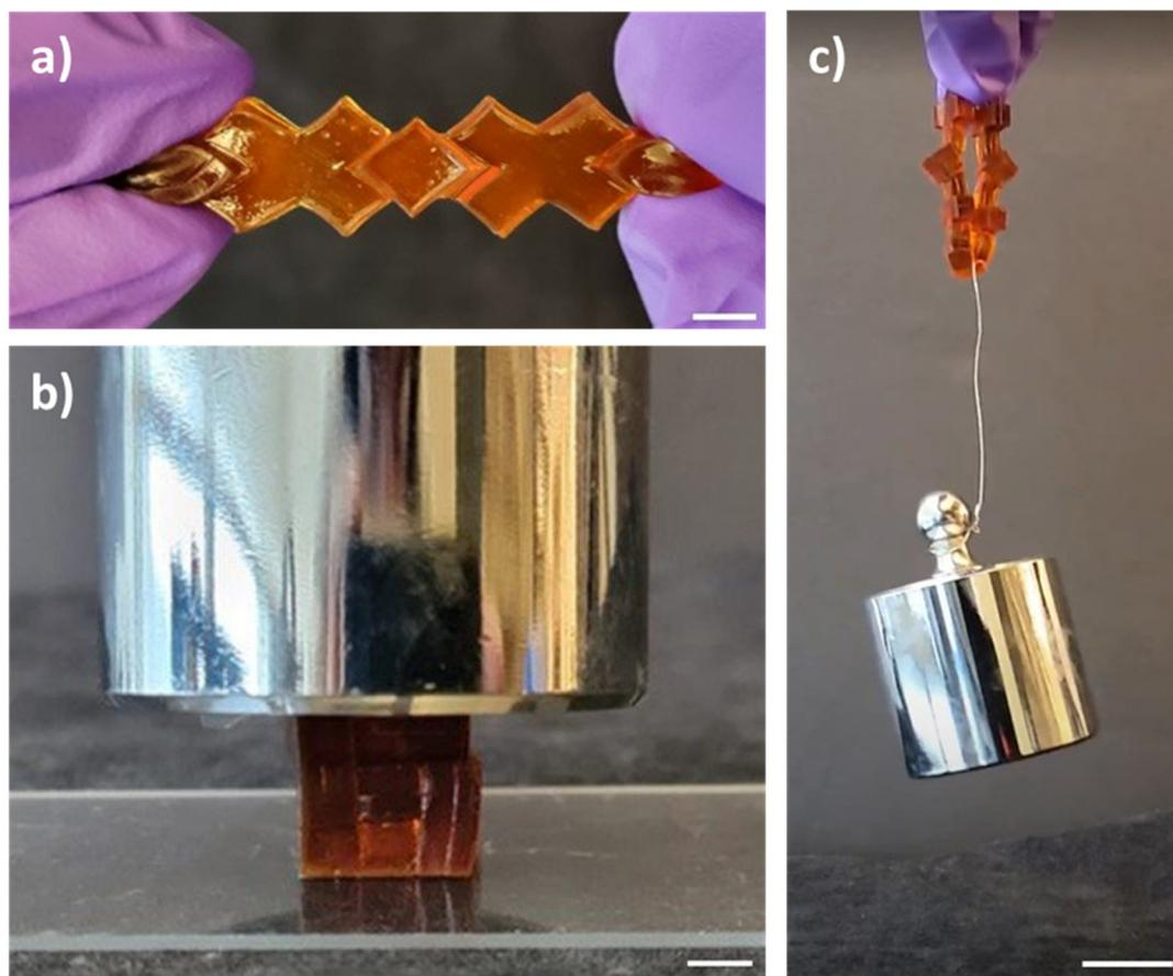
**Fig. 4** Demonstration of the mechanical robustness of assembled and fused piezoionic sensors as a (a) linear, (b) box, and (c) loop. The weight shown is 500 g. The scale bar for linear and box structures represents 5 mm. Scale bar for loop represents 20 mm.
