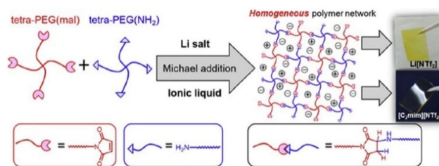
Fig. 24 Formation of polymer electrolytes with a homogeneous PEG network via Michael addition reaction and containing either Li[N(Tf 2 )] or [C 2 mim][NTf 2 ]. Reproduced from ref. 204 with permission from Elsevier, Copyright [2019].
