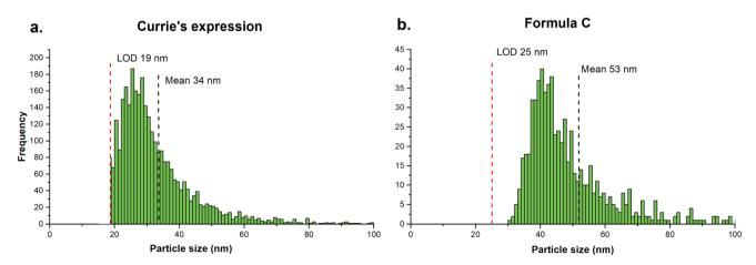
Fig. 4 Comparison of particles size distribution plots obtained by data processing using Carrie's expression (a) which counted 3191 particles and Formula C (b) which counted 696 particles.
