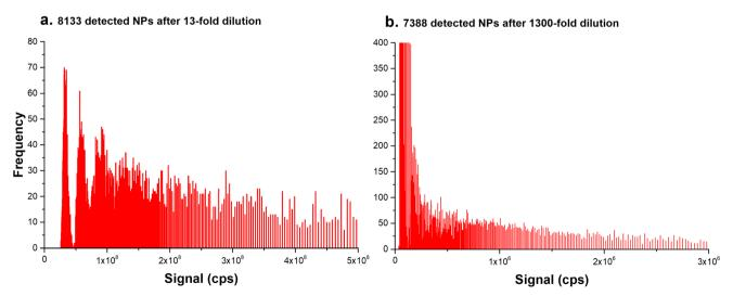
Signal distribution of Cu detected in sample 8 (a) after a 13-fold dilution, and (b) after an additional 100-fold dilution.
