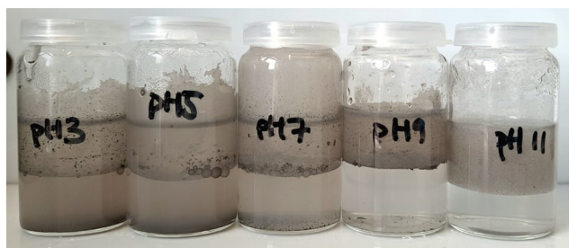
Fig. 5 NiO particle suspensions in two immiscible liquid systems (top: cyclohexane, bottom: DI water at different pH values). From left to right, pH 3, 5, 7, 9, and 11.
