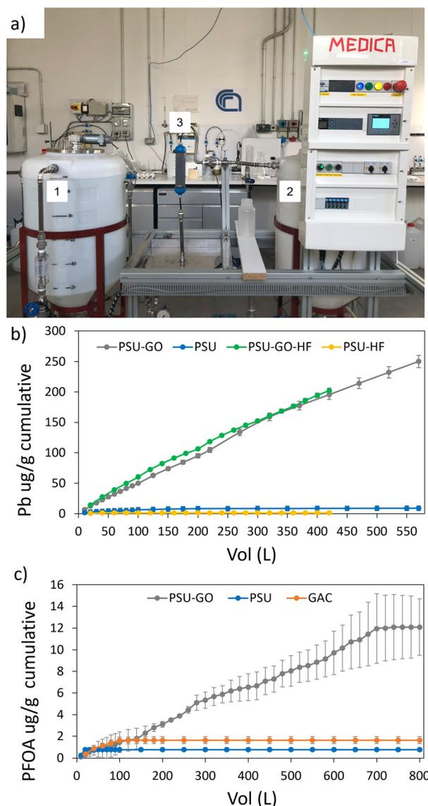
**Fig. 6** a) Set-up of the pilot plant used in this work. The pilot is connected directly to the tap. Spiked water in tank 1 (100 L capacity) is filtered through the cartridge (PSU-GO in the picture, filter 3) and filtered water is collected in tank 2 (100 L capacity). After 100 L are filtered, water is pumped from tank 2 to tank 1 (bypassing the cartridge) and the concentration is checked and adjusted to the target initial value. b) and c) Comparison between removal capacity on Pb and PFOA.
