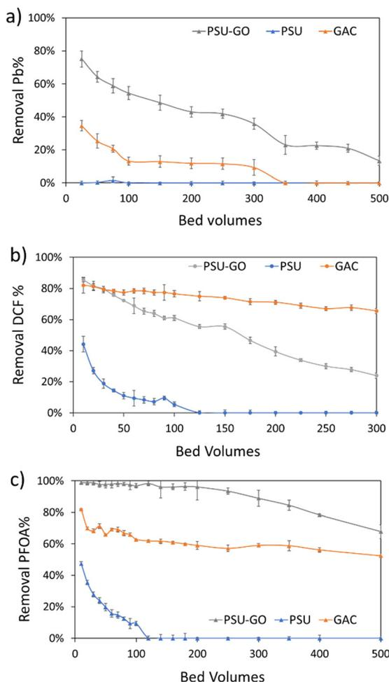
**Fig. 5** Loading curves of a) Pb, b) DCF, and c) PFOA expressed as removal % vs. bed volumes of PSU (blue lines), PSU-GO (grey lines) and GAC (orange lines). Full results are reported in Fig. S15, ESI†
