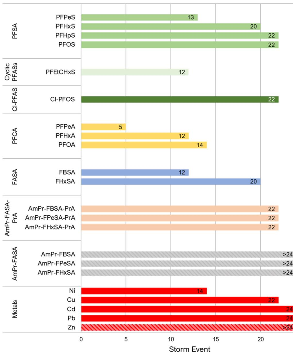
Fig. 3 Mean 10% breakthrough ( $C/C_0 =$  or  $>0.1$ ) storm event (storm event = 4 L; 95th percentile storm event at a relevant military site in Seal Beach, CA, USA) in unsaturated columns only, in order of chain length for select target and suspect PFASs and metals, grouped by contaminant class.
