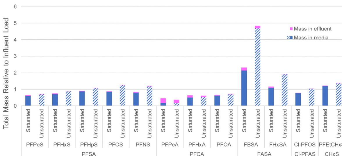
Fig. 5 Mass balance. The ratio of soil and effluent sums of mass loads to the total influent mass load in each condition; a value of 1 means the total mass load in influent is equal to total recovered PFASs in effluent and media. Mass in effluent was calculated by summing all mass in all samples measured with linearly extrapolated masses from storm events that were not assessed. Mass in filter media was calculated by multiplying the media concentrations by the column mass.
