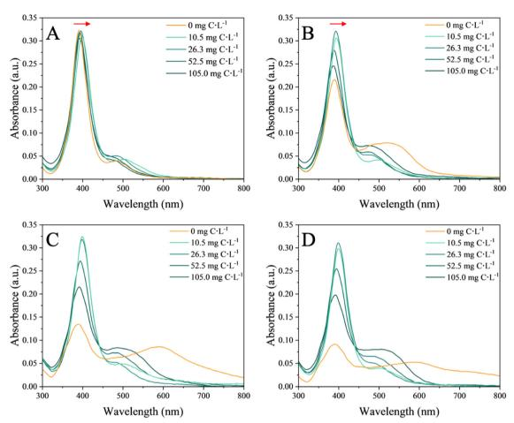
Fig. 1 UV-vis absorbance spectra of 4 mg L<sup>-1</sup> nAg in the absence and presence of increasing concentration of EPS (10.5, 26.3, 52.5, 105.0 mg C L-1) at the different incubation times: (A) 2 min, (B) 2 h, (C) 24 h and (D) 72 h. SPR characteristic peak of nAg is observed at 392 nm. The red arrows in (A) and (B) represent the red shifts.
