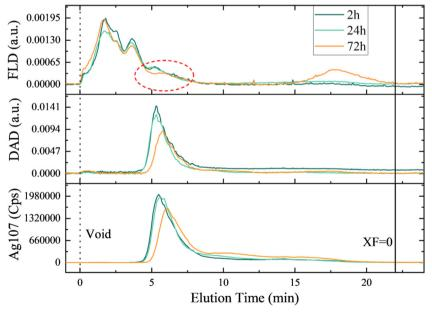
Fig. 7 Fractograms of 4 mg L<sup>-1</sup> nAg in presence of 26.3 mg C L<sup>-1</sup> EPS at different time points obtained by the AF4-DAD-FLD-ICP-MS. the signals originate from different detectors: Aq<sup>107</sup> from ICP-MS, DAD represents absorbance at 394 nm for nAq SPR and FLD is the fluorescence for protein tryptophan-like fluorophores. The red circle represents the formation of new peak (or bump) in protein signal coeluting with of the nAg.
