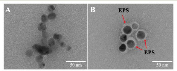
Fig. 4 Illustration of the formation of the EPS corona on nAg. TEM images of 4 mg L<sup>-1</sup> nAg in the absence (0 mg C L<sup>-1</sup>) (A) and presence of 105.0 mg C L<sup>-1</sup> EPS (B) incubated for 2 h. Sample were stained with uranyl acetate.
