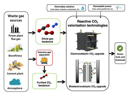
Fig. 1 Overview of emerging  $CO_2$  capture and conversion pathways. Proposed process flow for electrified  $CO_2$  conversion with selection of waste gas feedstock, omission or inclusion of gas separation device, and choice of  $CO_2$  conversion nanotechnology.
