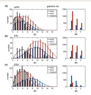
Fig. 3 Number distribution of oxygen (left) and nitrogen (right) in fresh (black), short aged (blue) and medium aged (red) gasoline car emissions for each ionization technique (a: APPI, b: ESI-, c: ESI+).
