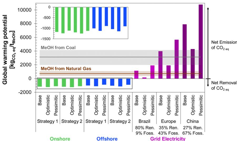
Fig. 13 Global warming potential (GWP), quantified as  $\text{kg}_{\text{CO}_2\text{eq}}$  per  $t_{\text{MeOH}}$ , for DAC-PtM under all investigated wind-powered scenarios, compared against DAC-PtM driven with grid electricity (mix of energy sources) from Brazil, Europe, or China.
