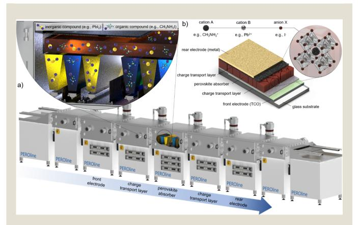
Fig. B1 General concept of vapor processing of perovskite solar cells. (a) Concept for the in-line fabrication of fully vapor-processed perovskite solar cells together with the general processes taking place during the co-evaporation of organic and inorganic compounds (see enlarged detail). (b) Sample layer stack sequence for opaque perovskite solar cells.
