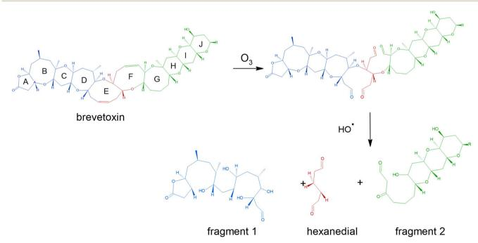
Possible fragmentation products of brevetoxin with its reaction with O<sub>3</sub> and 'OH.
