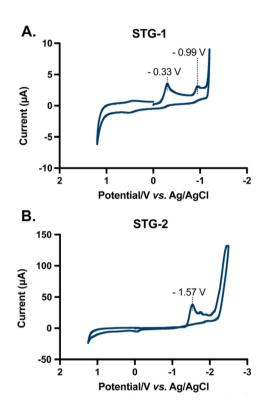
Fig. 3 Cyclic voltammograms of STG compounds (5 mM) in DMSO with [N(Bu)<sub>4</sub>PF<sub>6</sub>] as supporting electrolyte. Potentials are shown vs. Ag/ AgCl. (A) Voltammogram of STG-1 showing two reduction events at -0.33 V and -0.99 V. (B) Voltammogram of STG-2 showing one reduction event at -1.57 V. Data collected with a glassy carbon working electrode and Pt counter electrode.
