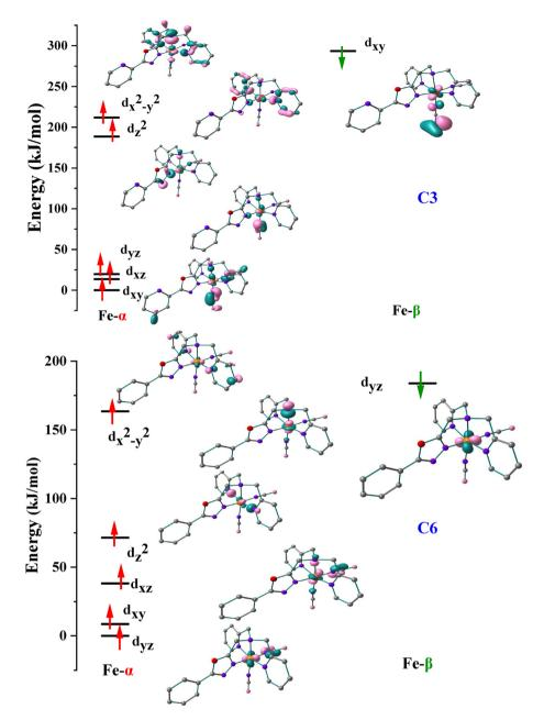
Fig. 9 Eigenvalue plot computed for C3 and C6. Here,  $\alpha$  and  $\beta$  represent spin-up and spin-down configurations. The energies are scaled to the lowest spin-up orbitals in each case.
