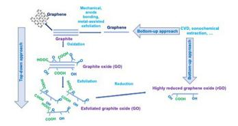
Fig. 3 Preparation of graphene derivatives, graphene oxide and reduced graphene oxide.
