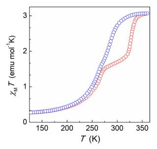
Fig. 2 Variable temperature dc magnetic susceptibility ( $\chi = M/H$  per mole of compound) data for 1 from 125 to 360 K, collected at 3 K min<sup>-1</sup> under an applied field of 0.5 T. Cooling and heating modes are shown in blue and red, respectively.
