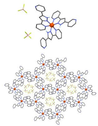
Fig. 1 Representation of  $[Fe(HL)_3](BF_4)_2$  (1) (top) and the crystal packing along the c axis (bottom). Fe, N, C, B, F and H atoms are shown in orange, blue, grey, pink, green and white, respectively. Only H atoms from the pyrazolyl NH groups are shown for clarity.
