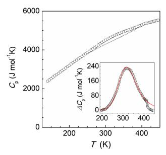
Fig. 5 Molar heat capacities of compound 2. The dashed line represents the estimated normal heat capacities used for  $\Delta C_n$  determination. Inset: excess heat capacity and its simulation using Sorai domain model (see text).
