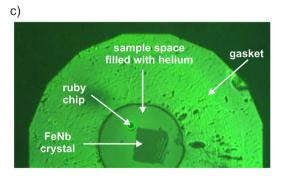
Fig. 1 Structural diagrams showing the molecular fragment of FeNb with the Fe<sup>II</sup> coordination sphere labelling scheme (a) and the packing diagram along the c direction (b). H and O atoms are omitted for clarity. Fe - orange, Nb - cyan, C - grey, N - blue. Picture of the FeNb single crystal inside the membrane DAC (c).
